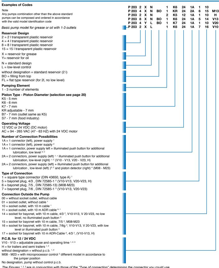
The Figures 1.2.3 are in conjunction with those of the "Type of connection" determining the connector you could use
